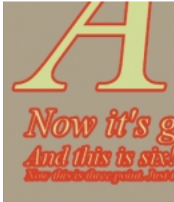
Figure 9: Trapping without small object protection
